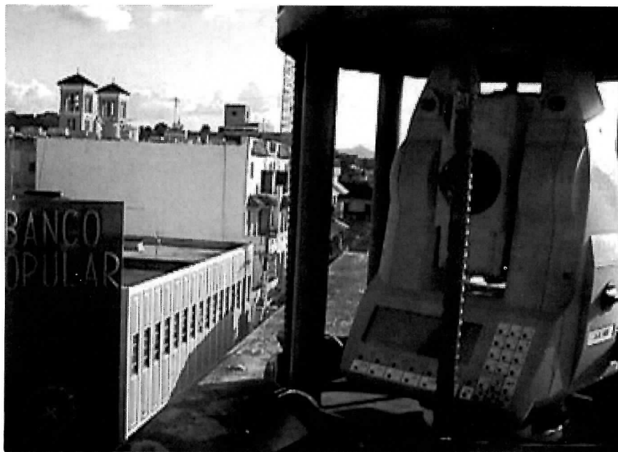
Figure 5. Motorised theodolite on building roof
